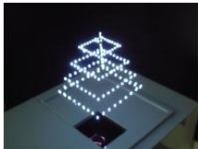
Figure 6. A 3D-object displayed using a 3D-image spatial drawing device. Credit: National Institute of Advanced Industrial Science and Technology.
